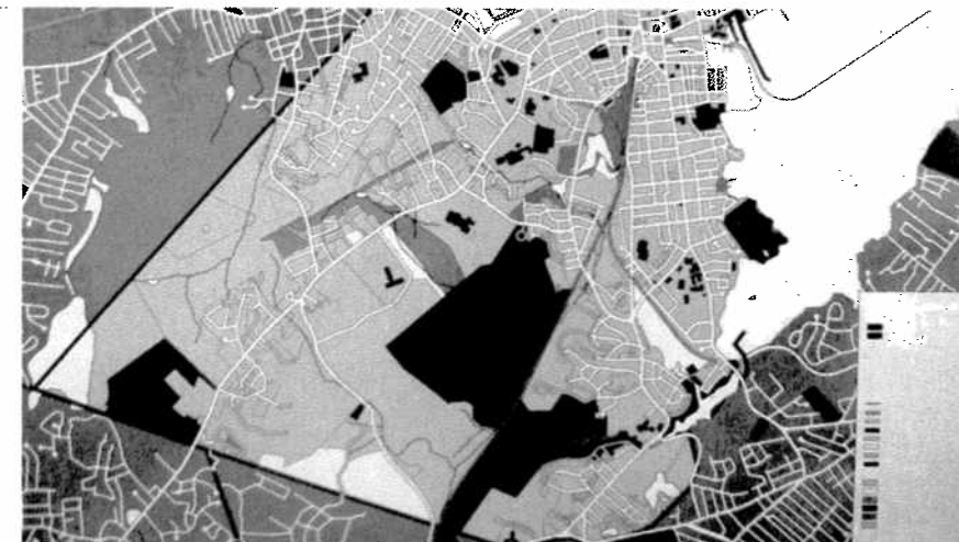
Figure 2a: Screened Scitex film containing all the yellow color for a four-color map.
