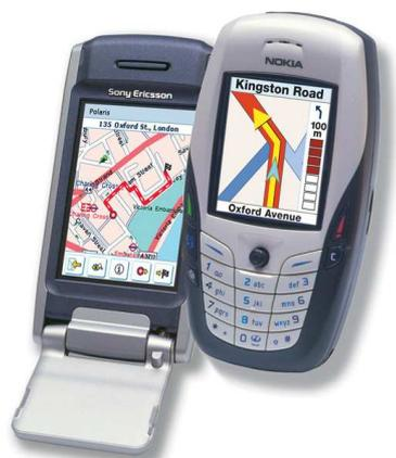
The **Polaris** system by Telmap (Herzlia, Israel) takes off-board navigation one step closer to its on-board predecessor. In addition to turning manoeuvres and voice instructions, Polaris offers full-colour maps that are tailored to the device being used. On an iPAQ, for example, with a high resolution colour screen, the maps are rich and detailed, similar to the best high-end autonomous systems. On a Java-enabled mobile phone, the detail is reduced to improve clarity
