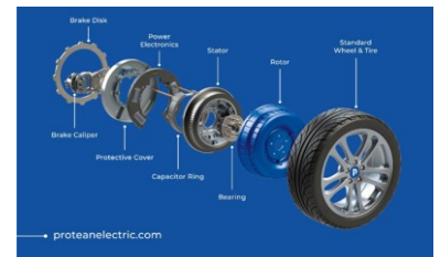
Protean Electric's in-wheel motor
