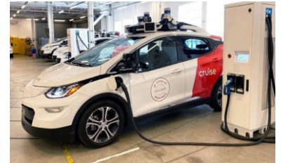
The current Cruise vehicle is a modified version of the Chevy Bolt Electric Vehicle.
