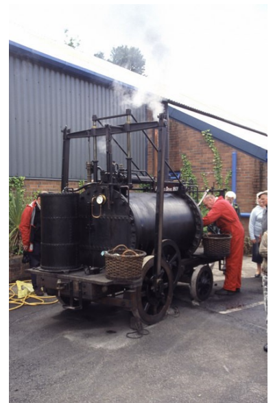
This is a replica of Trevithick's Puffing Devil, built by the Trevithick Society in Cornwall. It is arguably the first operational automobile. While French Army Captain Nicolas-Joseph Cugnot in 1770 built the first full-size working self-propelled mechanical land vehicle, also driven by a steam engine, the three-wheeled vehicle was very unstable and its engine was not up to the task of propelling the 2.5 ton contraption.
