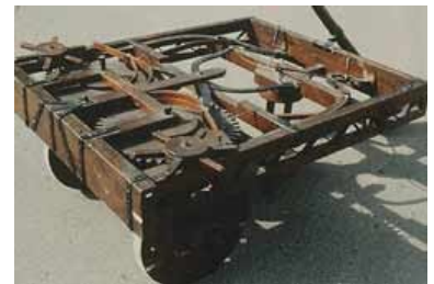
Da Vinci's designs for a self-propelled vehicle moved by the interaction of springs with geared wheels. Image: Courtesy of Museo Nazionale della Scienza e della Tecnologia Leonardo da Vinci
