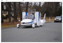
The model pictured above is called The Transition and is billed by the company as "the world's first practical flying car." The company says it runs premium unleaded petrol, fits into a standard single-car garage and converts between flight and drive modes in under a minute. You'll need a Sport Pilot Certificate to lift off the ground, but you can drive it around town with a regular driver's
