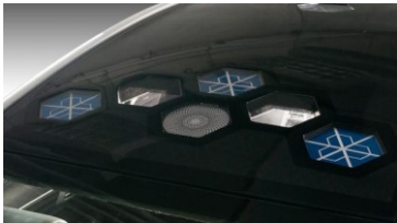
Six-sided antennas fit into receptacles on the roof of Toyota's Mirai concept car. (Credit: Kymeta)
