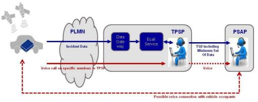
The first objective of TPS-eCall is to transfer an emergency message (incident data) from a vehicle to a TPSP in the event of a crash or an emergency situation, and to establish a voice channel between the in-vehicle equipment and the TPSP.
